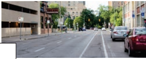
Paint only; cyclists can enter/exit anywhere but are vulnerable to car traffic
